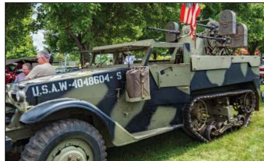
WW II 21 foot long, 10-ton M16 Multiple Gun Motor Carriage half-track, mounting quad .50 caliber machine guns as main armament
